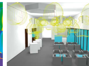
The LIDC gives the designer a hint about the resulting effect of the lighting.
