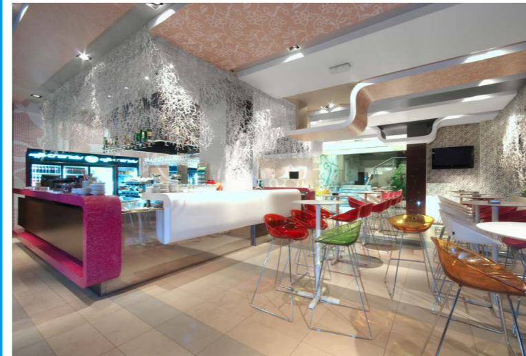
Since the luminaires placed directly above the self-service counter are exposed to a higher steam concentration, it is better to use those of protection class IP 65.
