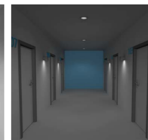
During times when the frequency of movement within a corridor is expected to be higher, it is possible to use presence detectors to dim the lighting to a reduced level for brief periods when nobody is around. These intervals are short but can still provide considerable energy savings over time.
