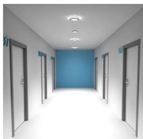
It is better to use various levels of illumination to provide visual cues as to where visitors are and to suppress the feeling that they are walking along a never-ending corridor.
