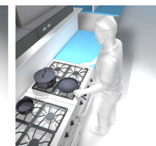
Illumination from above and slightly to the left of the workspace reduces the occurrence of shadows across the task area
