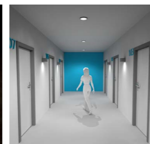
Most corridors have little or no access to daylight and require 24 hour illumination. LED light sources are an efficient and effective solution.
