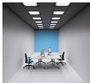
It is not advisable to use luminaires providing only direct distribution of the luminous flux because they do not create sufficient vertical and horizontal illuminance and result in a 'cave effect', which makes employees feel cramped and claustrophobic.
