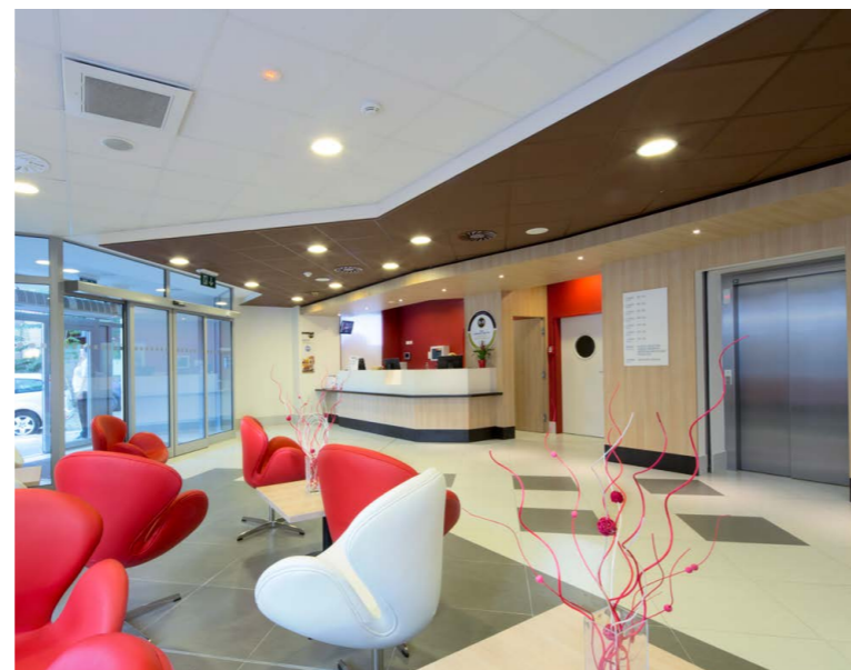
The European standard EN 12464-1 defines a minimal illumination of 300 lx and a lighting uniformity of 0.6 at the reception desk. Light sources must ensure a glare factor of no more than UGR 22 and provide colour rendition of at least CRI ≥ 80.
